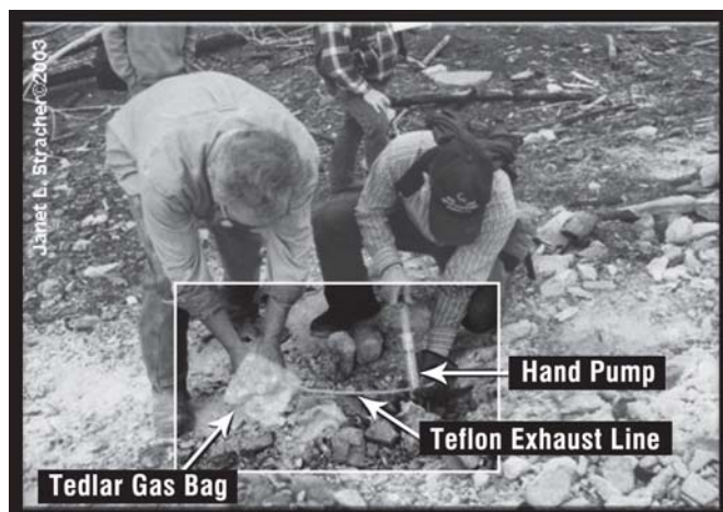
Figure 5. Collecting coal-fire gas, Centralia PA. Glenn Stracher (right) pumping coal fire gas from a vent through a Teflon exhaust line into a Tedlar gas collection bag held by Joe Nolter (left). The intake line in Stracher's left hand (leather glove) extends several cm down into the gas vent. Vent temperature measured with a thermocouple was 363 °C.
