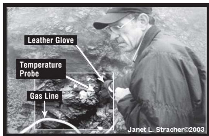
Figure 2. Hazards associated with collecting coal fire condensates and gas. Glenn Stracher is holding his breath to avoid inhaling toxic fumes. Note the lined leather glove used to protect his right hand during insertion of a thermocouple temperature probe into a coal fire vent: adjacent to a closed section of Route 61 on the eastern end of Centralia, PA. The white Teflon tube near the bottom of the photo was used to extract gas out of the vent with a hand pump). Gas temperature was 126.2 °C. CO and CO 2 , measured with Drager tubes, were highly toxic at 1000 ppm and 2200 ppm respectively. Condensation products associated with this vent have yet to be identified.
